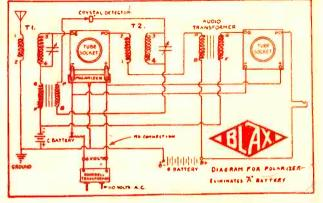
the Polarizer, instead of attaching them tto the glament lead. An ordinary 6 to 10 volt door bell transformer which has been connected to the electric lighting circuit is attached to the regular "A" binding posts. If desired, the same transformer in use for the residence bell may serve for this purpose. Blax Polarizer is manufactured in Los Angeles, but is being shipped to all
